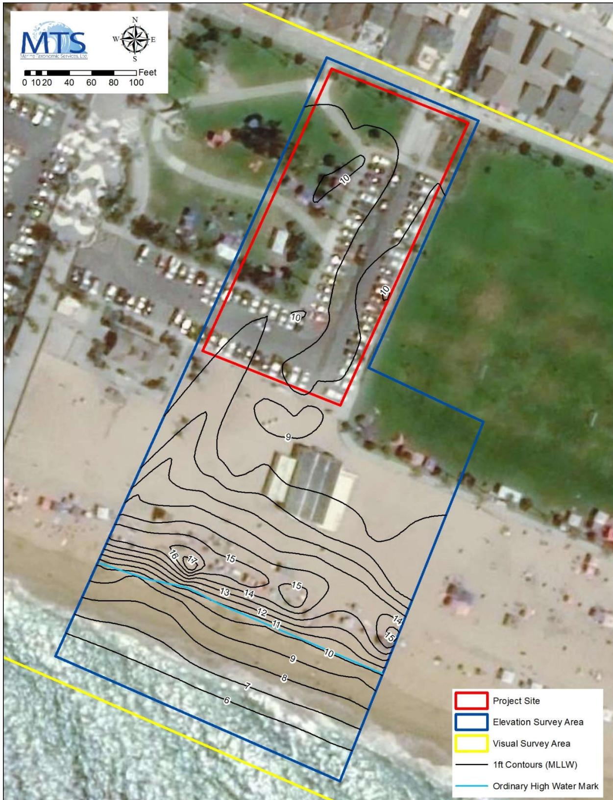
Figure 3. Map of elevation survey results delineating the Project site in Newport Beach. Data provided for habitat assessment purposes. Not intended to replace a certified land survey and not intended for navigation.
